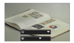
2. Two sliders will appear at the bottom of the screen to help users adjust the live view to suit the ambient lighting conditions being used. The top slider is a speed vs. quality slider. Increase the quality by moving slide to the right or achieve a faster frame rate on the left. The lower slider controls the brightness of the Live View.
