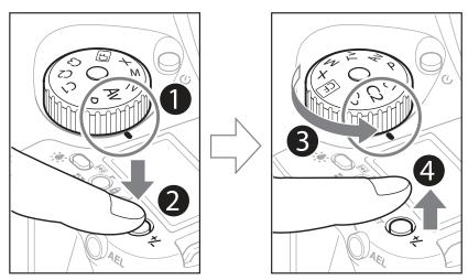
\*The illustration shows the exposure mode Av (aperture priority AE) being recorded to C2.
