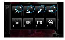
The Full Screen Context Menu features a Delete/Rating, Exposure Warning, Custom White Balance Picker and Grid options. Press and hold these icons (with a white triangle in the corner) to further configure.
