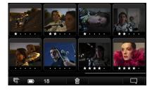
The Thumbnail View displays all images stored on a CompactFlash card in a series of 8 thumbnails.
