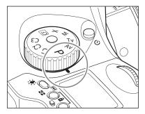
P: Program AE - The aperture and shutter speed are determined automatically for the optimum exposure, according to the ambient light conditions. This auto mode is best suited for general photography or for novice photographers, as it leaves the user free to concentrate on framing and capturing the subject.
