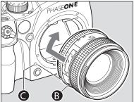
2. Align the white alignment dot of the lens [B] (on the shiny flange) with the camera's white dot [C]. Mount the lens and rotate it clockwise until it clicks into place.
