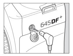
Flash Photography with Electronic Flash Models other than Metz units 1. To use a grip type flashgun or a strobe with other electric contacts than X contact, connect the sync cord to the camera's sync terminal. (See note below about flashes designed exclusively for other makers' cameras.)
